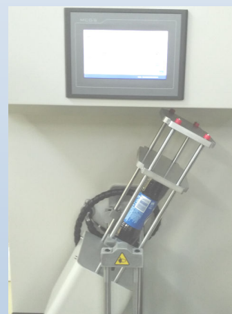
PET Bottle Carbonatoin Testing
