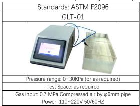
**Micro Leak Tester** is based on vacuum decay method, and is a non-destructive way for leak testing of rigid and semi-rigid non-lidded trays; trays or cups sealed with porous barrier lidding materials; rigid, nonporous packages; and flexible, nonporous packages.
